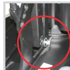
Remove the Handle Mounting Pin w/o Tools
