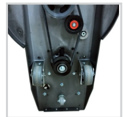
V-Belt Drives Pads at 2000 RPM
